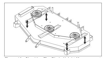
Figure 12. Checking The Blade Height Measurement
